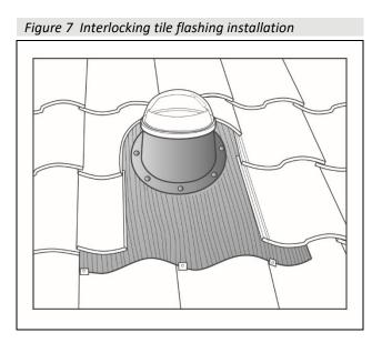
17.5 The top tube assembly is inserted into the roof flashing from the outside. Metal roof flashings have pre-drilled holes. The dome ring fixing holes align with these holes and dome screws are screwed through to the flashing to hold the top tube assembly temporarily in place.
