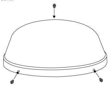
Fasten the dome with the dome screws supplied. Screw from the outside to the inside, through the spacers. Drive the screws through both the roof flashing and the reflective tube. Do not overtighten the screws or you may cause damage to the roof dome.
