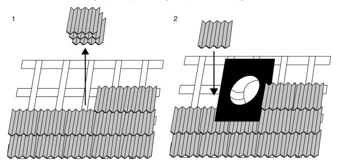
Create a weather stop by folding the sides and top of the flashing upwards by a few centimetres.
