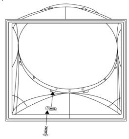
Carefully push the Natural Effect Lens up into the recess in the top of the transition box. Turn the white tabs a quarter turn to secure the Natural Effect Lens into place.
