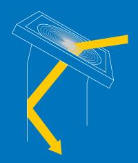
The new Solatube 35 cm  $\varnothing$  low profile roof daylight collector option replaces the roof dome and has the subtle appearance of a traditional skylight.
